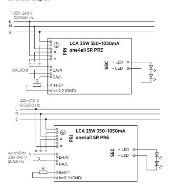
Device with loop through wiring function.
